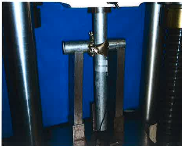
Photograph of setup for Indentation Check
