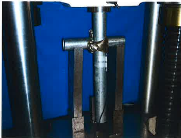
Photograph of Setup for Slipping Force
